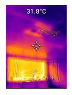
This image shows significant heat entering through an unshaded bathroom window. It can also be observed that the frame directly above the window has no insulation fitted at all. The room also has a heat lamp and extraction fan fitted to the ceiling. In this example insultation has been removed around the heat lamps.
