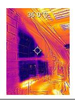
This image shows a kitchen window from outside of the home. By using external window shades, direct sunlight inside the home can be minimised. This reduces solar gain and keeps temperatures in the room cooler than outside on a hot day.
