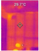
This image shows a section of wall in a bedroom area. The wooden frame and battens are clearly visible. Unlikely the insulation levels installed during construction are sufficient.
