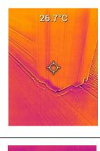
This image shows a wall where the floor has dropped, leaving a gap at the base of the wall, allowing cool air in and creating this darker, colder area at the base of the wall.
