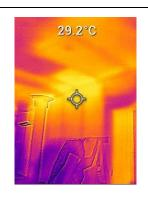
This image shows sections of wall and roof that have insufficient areas of insultation or sarking fitted. The majority of heat in the home is lost through the ceiling, top of walls and window areas.
